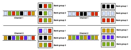
(a) No partition is used (cache-line interleaving) (b) BMP+ is used (BPM+ includes BPM) Figure 4. Interference elimination via BMP+.
