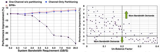
Figure 5. The correlation between bandwidth demands and performance changes caused by different policies. (This figure includes tens of workloads. The baseline is channel interleaving).
