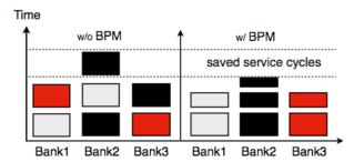
Figure 3. The comparison between interleaved address mapping and BPM. Different colors represent requests from different threads.
